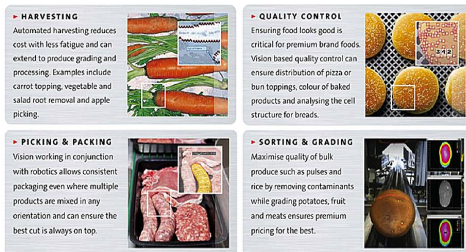
Figure 4 – AI and computer vision driven food industry (harvesting, picking, quality control and sorting)
