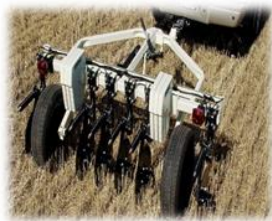
Figure 8 – Example of electromagnetic sensor: Veris EC sensor 84
